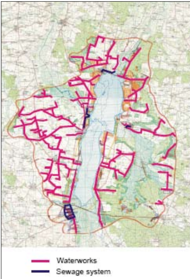
Fig. 5: The water-pipe and sewage network system on the Jeziorsko reservoir area.
